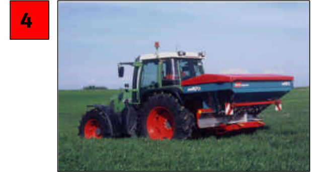
4 Either a static or a dynamic correction mode : The "real permanent weighing system with dynamic correction" of the spread rate during work. The static correction (after 200 kg) is advised when starting to spread a new fertiliser.
