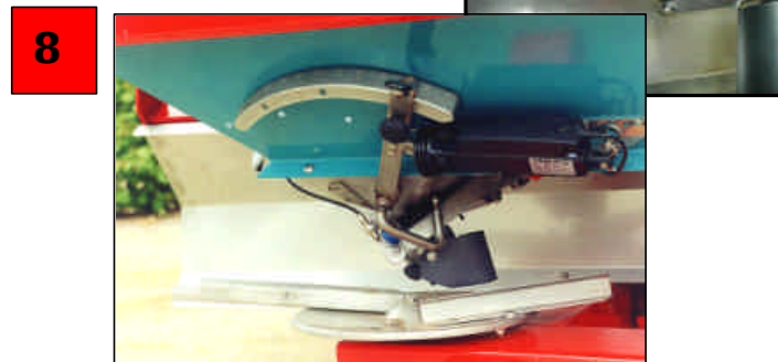
8 Double shutter control (hydraulic on/off + electric adjustment) : The Spreader remains independant from electronics. Whenever necessary, it is possible to return to manual settings in seconds thanks to the electric actuators. Shutter opening/closing is quick fit then instantly possible
