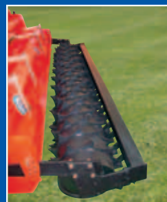
Rodillo Packer Rouleau Packer Packer roller
