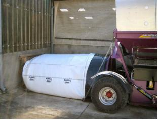
6. Lock the hydraulic brakes by pumping max pressure (about 150-170 bar) with the hand pump. Now crimper-bagger do not move forward during the start.
