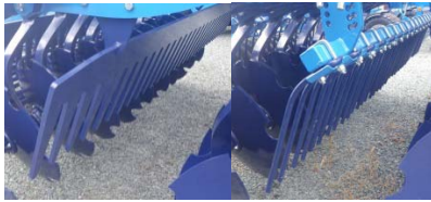
Selection of two types of deflectors ridge / comb
