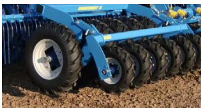
The double pneumatic-tyred roller allows lifting the rear roller, thus creating ridges causing the surface dry faster
