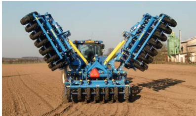
Patented folding system that allows folding the machine with the coverage of 7.8 m into the transportation width of 3 m and height of 4 m, which meets the regulations for operation on roads.
