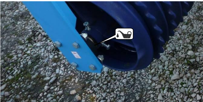
Fig.10 – Roller bearings lubrication
