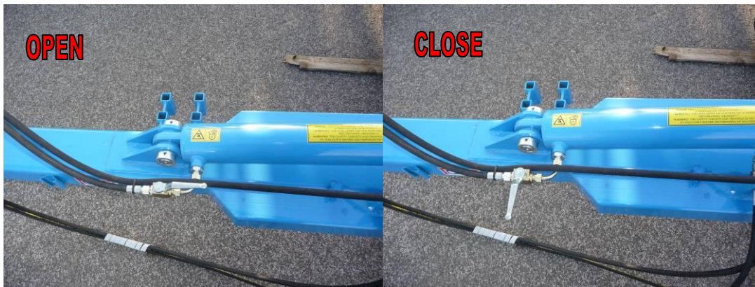
Fig. 5 – machine unfolding piston rod ball valve
