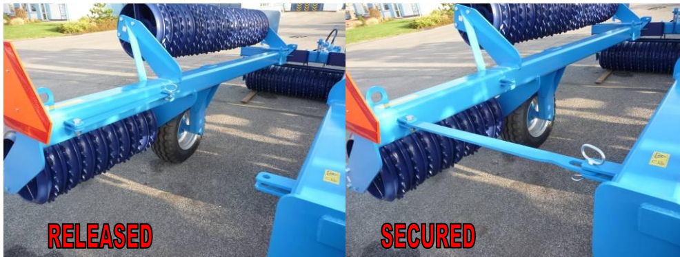
Fig.8 – connecting rod for side frames
