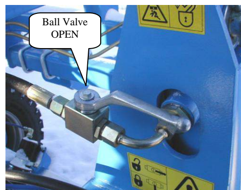
Fig. 6 - Ball Valve – OPEN
