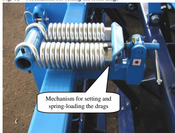
Fig. 12 – Mechanism for setting the front drags
