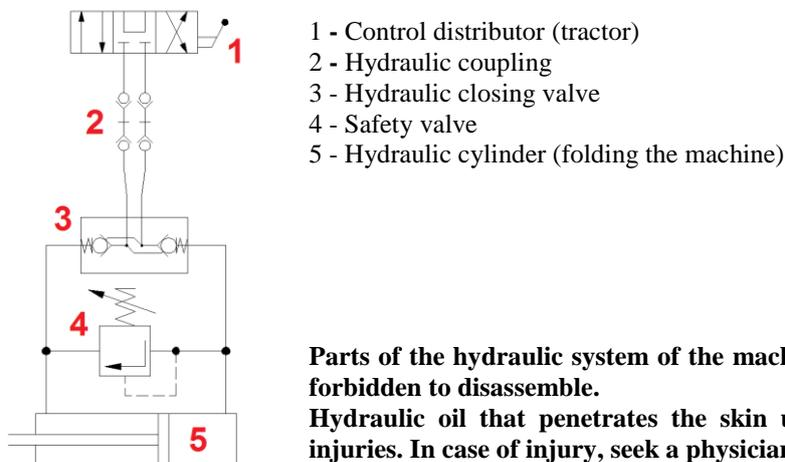
Parts of the hydraulic system of the machine, which are under pressure, are forbidden to disassemble. Hydraulic oil that penetrates the skin under high pressure causes severe injuries. In case of injury, seek a physician immediately.
