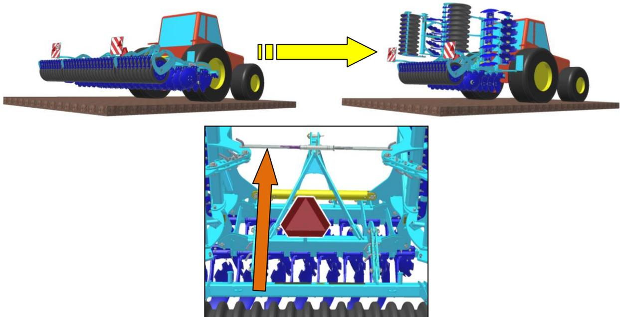
**Procedure for unfolding the machine into the working position**
