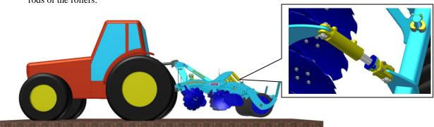
2. Retract the piston-rods of the rollers into the maximum top position (piston-rods are drawn in) so that the spacer rings placed on the piston-rods are compressed tightly. Place the machine in the tractor suspension on the ground. Set the longitudinal plane of the machine by adjusting the position of the bottom arms of the tractor and the drawbar of the third point of the tractor, thus ensuring the same working depth for both disc rows.
