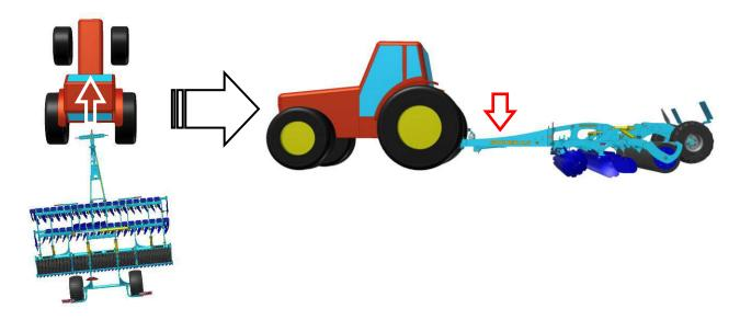
Fig.11 - When the machine turns to the left-hand side, lift the machine in arms
