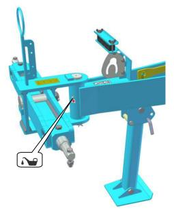
Fig.15- Rollers bearings
