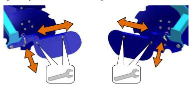
• The position of the edge discs is adjustable and they allow different recess against other discs. The adjustment is executed so that the working depth of the edge discs is lower (approx ½ - ¼ of the depth of the other discs) so that no unevenness is created on the land.
