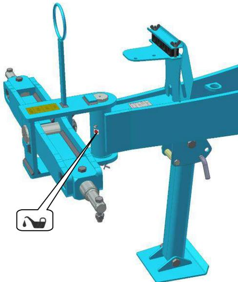
Fig.17 - Rollers bearings
