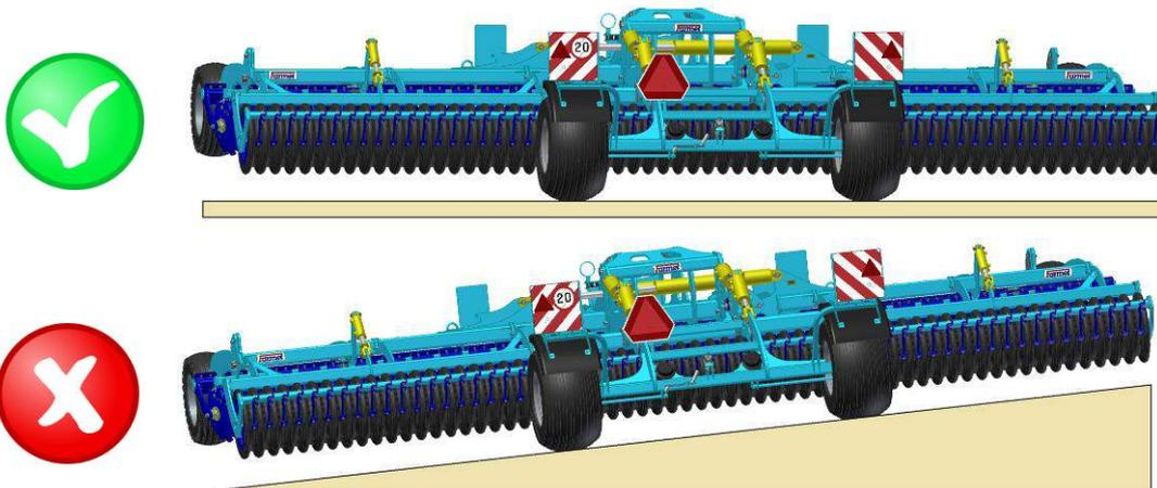
Fig.7 – Machine position for unfolding
