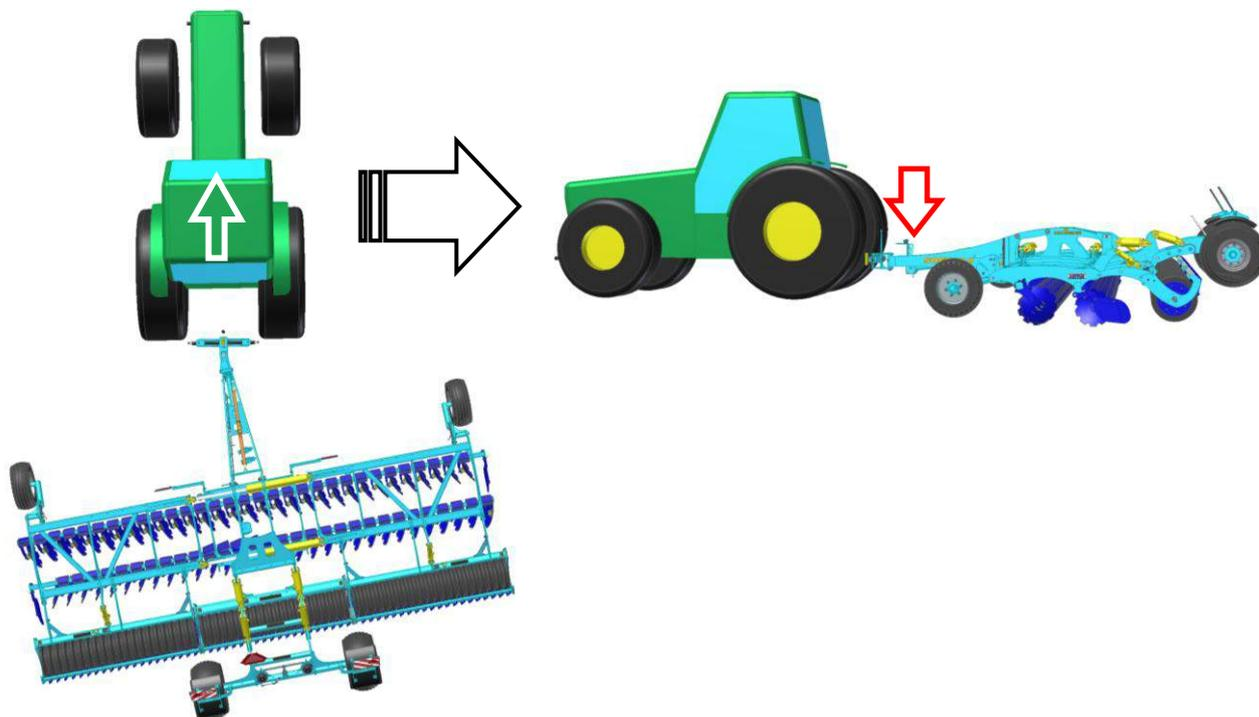
Fig.13 - When the machine turns to the left-hand side, lower the machine in arms
