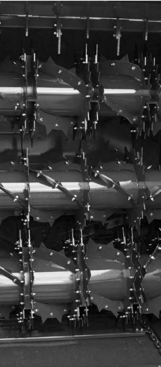
**BASIC and SMART proportional electric controls drive the moving floor with precision. Thanks to the SMART controls, the drive of the shredders regulates the moving floor speed depending on the distributed product.**
