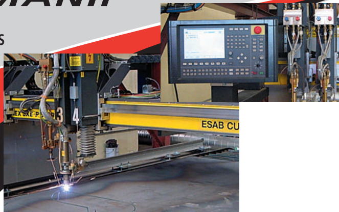
Oxycutting with numerical control.
