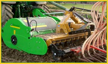
The Rotar digging machine is equipped with center drive (no chains in the machine!). With a direct PTO drive to the Alpego power harrow. The Alpego power harrow is integrated at the digging machine.
