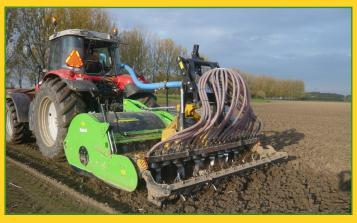
The Rotar digging machine in combination with a Alpego power harrow is a excellent tool for digging and drilling in one pass. The advantage is that you do not drive one the soil before drilling.
