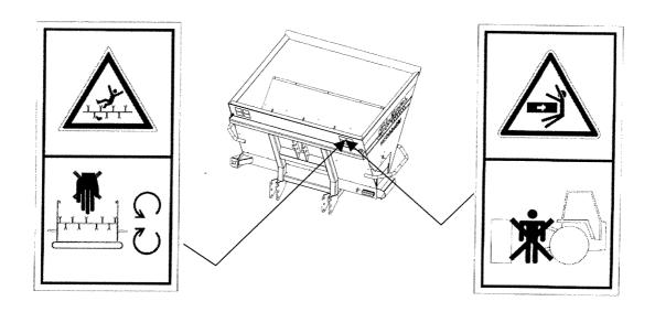
Risk of entanglement in agitator. Do not reach into Cubicle Bedder tub whilst engine is running on tractor/handler
