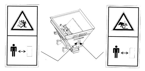
Thrown or flying objects. Keep a safe distance from Cubicle Bedder when machine is working
