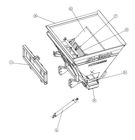
The machine can either be fitted to the three point linkage of the machine using a standard top link where by it must be loaded manually or from an overhead hopper. Alternatively a hydraulic top link can be supplied which alters the angle of the tub allowing it scoop bedding material form a bulk heap on the floor.
