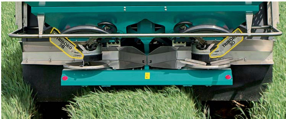
TRIBORD 3D border device available on the right-hand side (standard) AND left-hand side (option on ISOBUS versions)
