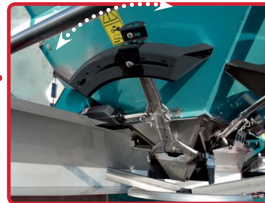
Electric setting from the cab (ECONOV version)
