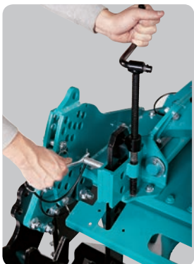
1 Rapid adjustment levelling board
