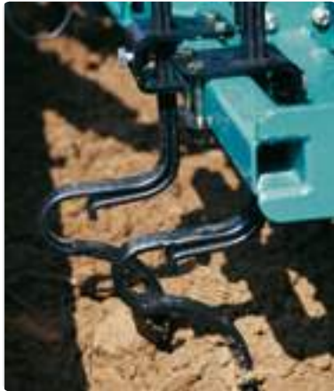
4-tine tractor wheel track eradicator (optional)
