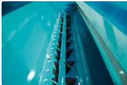
Hopper bottom with distribution cells giving ZERO «dead» volume, slow rotation agitator and retractable anti-compaction deflector giving a regular application rate whatever the load in the hopper
