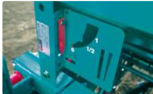
Indicators for hopper seed level, vertical position and tramlining
