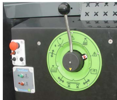
Induction hopper operating zone with multi way valves and TECFLOW (optional)
