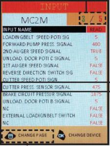
This sensor shows us on the ALGA TFT panel by the functions menu, the instant working pressure of the milling cutter. When the milling cutter is OFF, the display shows the boost pump pressure. On the diagnostics page of the **LOGICAL INPUT** MC2M will be reported the mVolt value of the pump.
