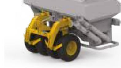
TASSE AVANT INTÉGRÉ (PNEUS 10.0/75 – 15.3 – DIAM. 740MM)
