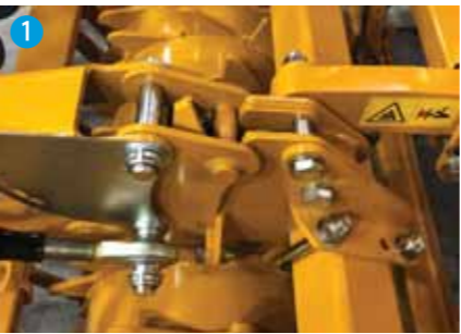
Quick release system of the seeding bar from the power harrow.
