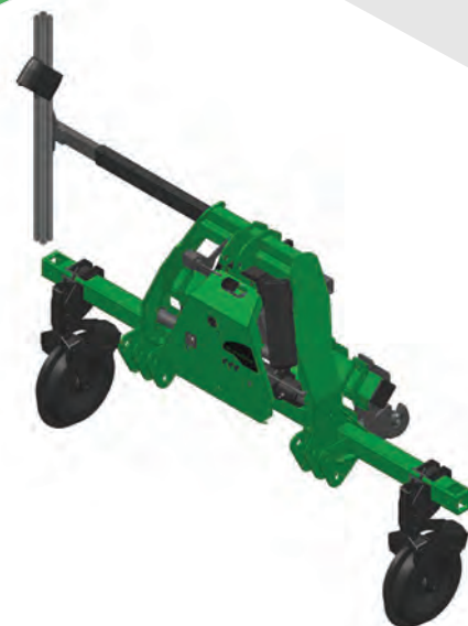
TRACKER Koppelframe met sideshift en camera TRACKER Driving system with camera
