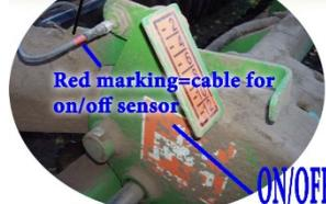
Red marking=cable for on/off sensor
