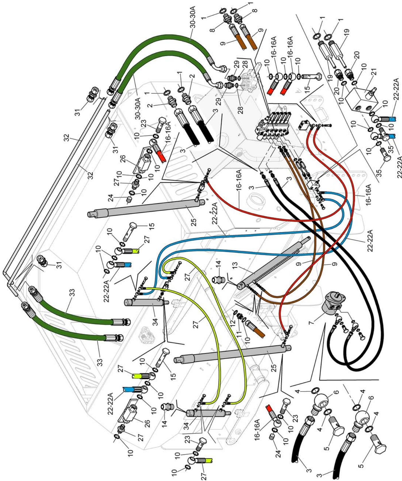
**IMPIANTO IDRAULICO STANDARD DS 9/12/16 m<sup>3</sup>**
