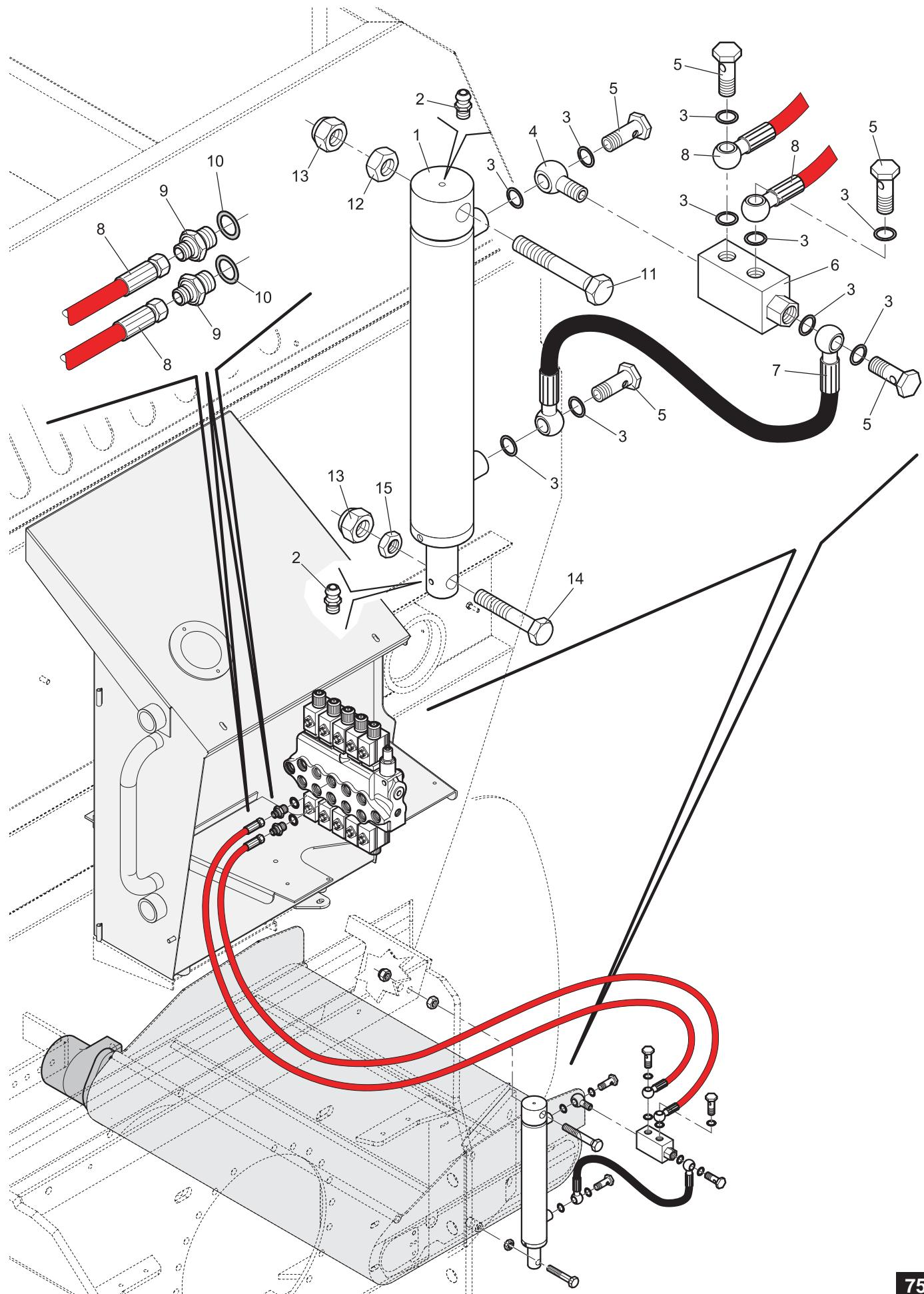
**(OPT) IMPIANTO SCARICO REGOLABILE DESTRO G 9/12/15 - 5/7m<sup>3</sup>****(OPT) SYSTEM UNLOADING RIGHTADJUSTABLE G 9/12/15 - 5/7m<sup>3</sup>****(OPT) ANLAGE AUSLADEN REGULIERBAR RECHTS G 9/12/15 - 5/7m<sup>3</sup>****(OPT) SYSTEME DE DÉCHARGEMENT REGLABLE DROITE G 9/12/15 - 5/7m<sup>3</sup>****(OPT) INSTALACIÓN DE DESCARGA AJUSTABLE DERECHA G 9/12/15 - 5/7m<sup>3</sup>****husky**
