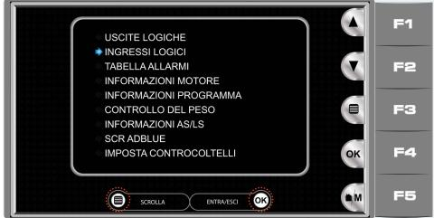
Press the "touch" key of the "scroll" booklet (part.1 fig.1) or the "F3" button (part. 2 fig.1/1) to move the blue arrow to the "LOGICAL INPUTS" item (fig.2).
