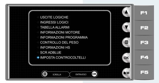
Press the "touch" key of the "scroll" booklet (part. 1fig.1) or the "F3" button (part. 2 fig.1/1) to move the blue arrow to the "SET COUNTER-BLADES" item (fig.2).
