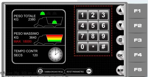
In the first figure (fig. 10) an are CAMBIA PASAN PESO RESET uct that is leaded into the chamber is displayed. The quantity of the visible weight (part.1 fig. 10) is the same as that seen on the weight in real time (only with CAN BUS weight).
