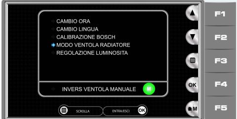
Press the "touch" key of the "scroll" booklet (part.1 fig.1) or the "F3" button (part. 2 fig.1/1) to move the blue arrow to the "RADIATOR FAN MODE" item (fig.2).
