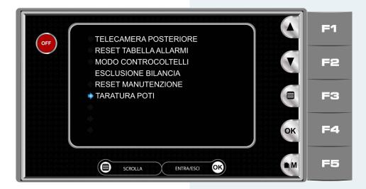
Press the "touch" key of the "scroll" booklet (part.1 fig.2) or the "F3" button (part.2 fig.2) to move the blue arrow to the "POTI CALIBRATION" item (fig.3).
