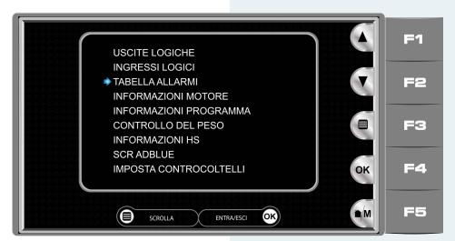
Press the "touch" key of the "scroll" booklet (part.1 fig.1) or the "F3" button (part. 2 fig.1/1) to move the blue arrow to the "ALARMS TABLE" item (fig.2).
