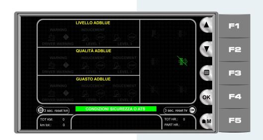
This page displays the icons of the types of inducement or regeneration present managed by the engine control unit.
