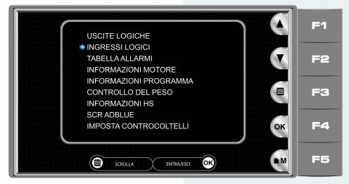
Press the "touch" key of the "scroll" booklet (part.1 fig.1) or the "F3" button (part. 2 fig.1/1) to move the blue arrow to the "LOGICAL INPUTS" item (fig.2).
