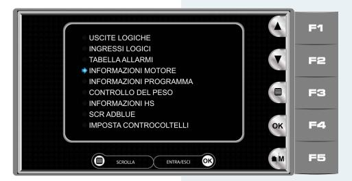
Press the "touch" key of the "scroll" booklet (part.1 fig.1) or the "F3" button (part. 2 fig.1/1) to move the blue arrow to the "ENGINE INFORMATION" item (fig.2).
