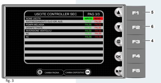
on these three pages, it is possible to see the utilities managed by the secondary control unit. The green text under the word "WRITE" must correspond to the red text under the word "READ".
