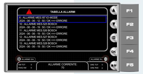
On this screen, all the current errors of all the control units of the machine are displayed.
