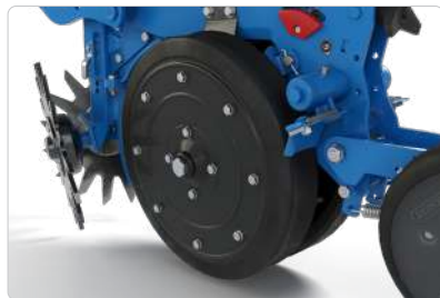
NARROW GAGE WHEELS DIAM. 50MM
